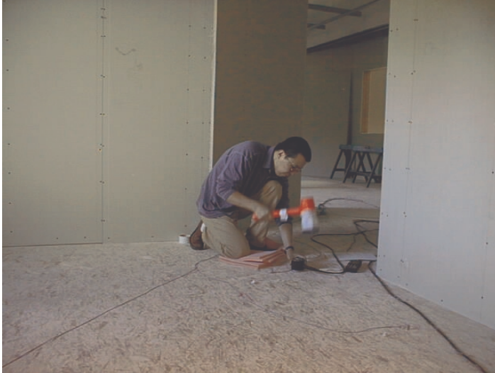
Figure 18: Hammer excitation of the floor.
